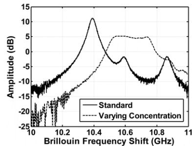
Fig. 2. Area normalized Brillouin gain spectra for standard and varying concentration phosphosilicate fibers.
