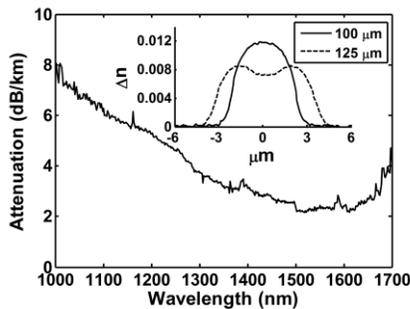
Fig. 1. Attenuation as a function of wavelength and refractive index profile (inset) for varying concentration phosphosilicate fiber.
